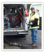
the street, a giant rodder and hydro-jetter are used. Sometimes, however, a thorough cleaning job needs to be done by hand. Here, Juan and the other crew members go down into the sewers and use hand tools to clear the lines. Toxic gasses, such as methane, carbon dioxide, and hydrogen sulfide are always potential problems that need to be checked for before venturing down into a main.
